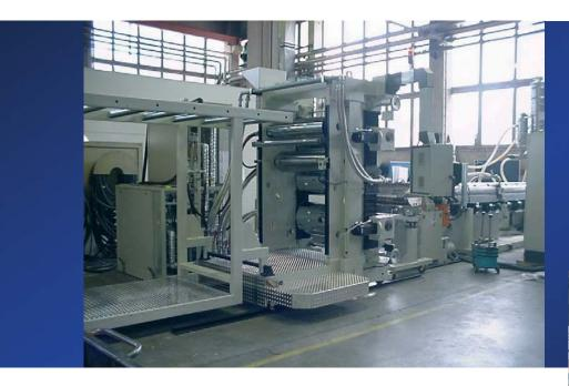
Our double-walled standard smoothing rollers, which can be used for all applications in the smoothing as well as the calendering unit, are fitted with an intermediate conductive coil and are hard chrome-plated. The roughness values of their polished surfaces are below  $R_t$  0.2  $\mu m$ .
